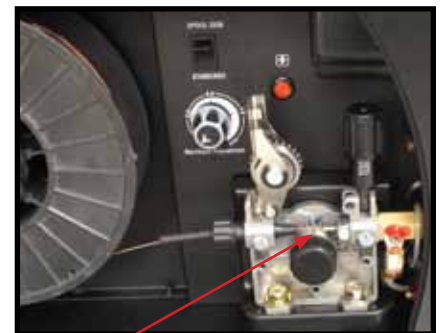
(8) Feed wire over the drive roller into the outlet guide tube, Push the wire through approx 5.9 Inches.
