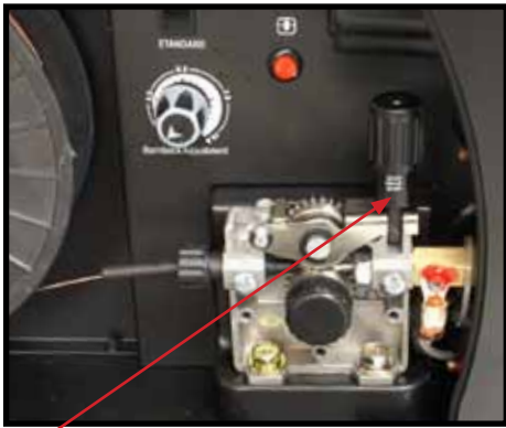
(9) Close down the top roller bracket and clip the pressure arm into place.
