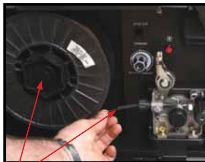
(7) Place wire onto spool holder - (spool retaining nut is left hand thread ) Feed the wire through the inlet guide tube on to the drive roller.
