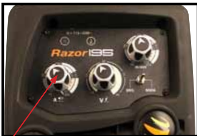
3) Set the welding current using the amperage control dial
