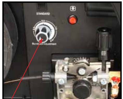
(17) Adjust the burn back control to prevent the wire sticking in the weld pool.
