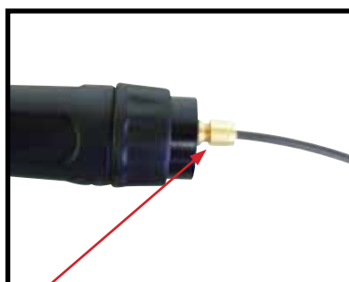
(8) Push the liner firmly into the torch lead and tighten the liner retaining nut
