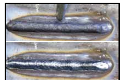
8) Wait for the weld to cool and carefully chip away the slag to reveal the weld metal below.
