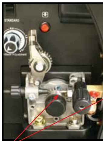
(6) Fit the correct sized Knurled Drive roller for Gas Less Flux Cored wire
