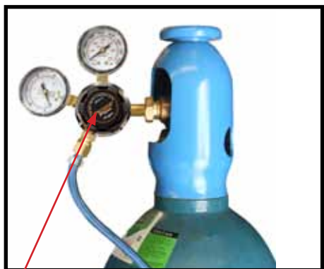
(15) Carefully open the valve of the gas cylinder, set the flow to 25CFH
