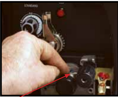
(8) Feed wire over the drive roller into the outlet guide tube. Push the wire through approx 5.9". Use a Knurled Drive Roller of the correct size
