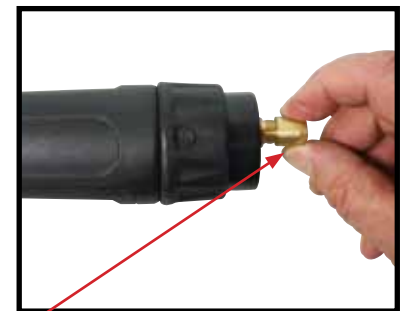
(6) Fit the liner retaining nut and screw only 1/2 way down
