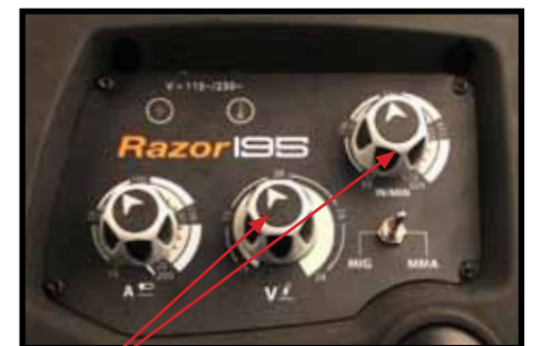
(20) Set welding parameters using the voltage and wire feed controls.
