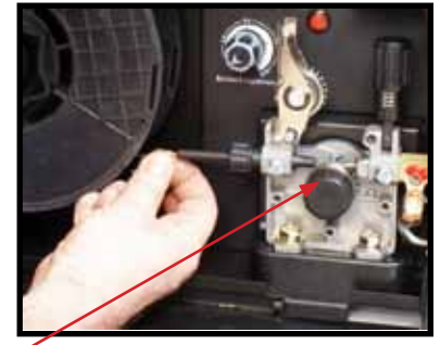
(7) Place aluminium wire onto spool holder. Feed the wire through the inlet guide tube on to the drive roller.
