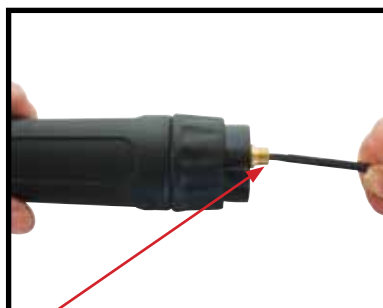
(5) Carefully feed in the new liner in short forward movements down the torch lead all the way to exit the torch neck. Be careful not to kink the liner
